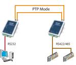
TX). To expand the number of connected serial devices users can apply the SFP configuration mode and connect the fiber transmitter to the rest of the slaves and eventually back to the master node.
