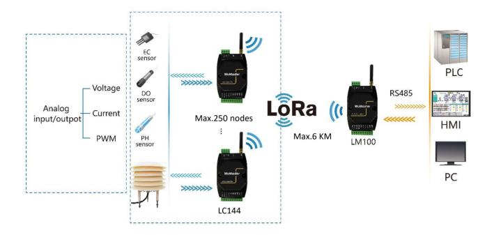
Transparent LoRa Communication to extend Two-Way Modbus Sensor Read and Control
