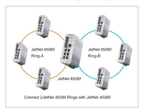
rings into a line or into multiple directions. In addition to extensibility, MultiRing<sup>™</sup> has great diversity of various ring technologies. When MultiRing<sup>™</sup> enabled, JetNet 4508if can connect RSR rings, TrunkRing<sup>™</sup> and a Super Ring together and simultaneously provide more Fast Ethernet Ring connectivities. This provides extensibility to new technologies while keeping the great backward compatibility.
