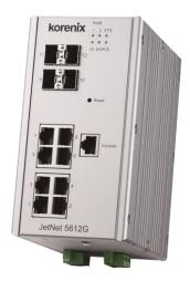
The JetNet 5612G-4F is an pure Gigabit industrial Ethernet Switch with 8 ports RJ-45, 4 ports Gigabit SFP socket for optical fiber network connection. It adopts high efficiency Ethernet MAC controller with 24Gbps Switch fabric bandwidth, 9K jumbo frame forwarding. The robust system design makes the JetNet 5612G-4F survive under harsh outdoor environment with extreme electric magnetic interference and the variation of environment temperature.
