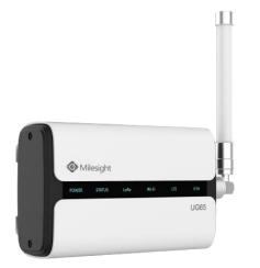
UG65 is a robust 8-channel indoor LoRaWAN<sup>®</sup> gateway. Adopting SX1302 LoRa chip and high-performance quad-core CPU, UG65 supports connection with more than 2000 nodes. UG65 has line of sight up to 10km and can cover about 2km in urbanized environment, which is ideally suited to smart office, smart building and many other indoor applications.
